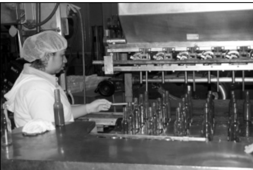
THIS MACHINE FILLS SIX TO EIGHT BOTTLES AT A TIME AT A RATE OF APPROXIMATELY ONE HUNDRED PER MINUTE.
